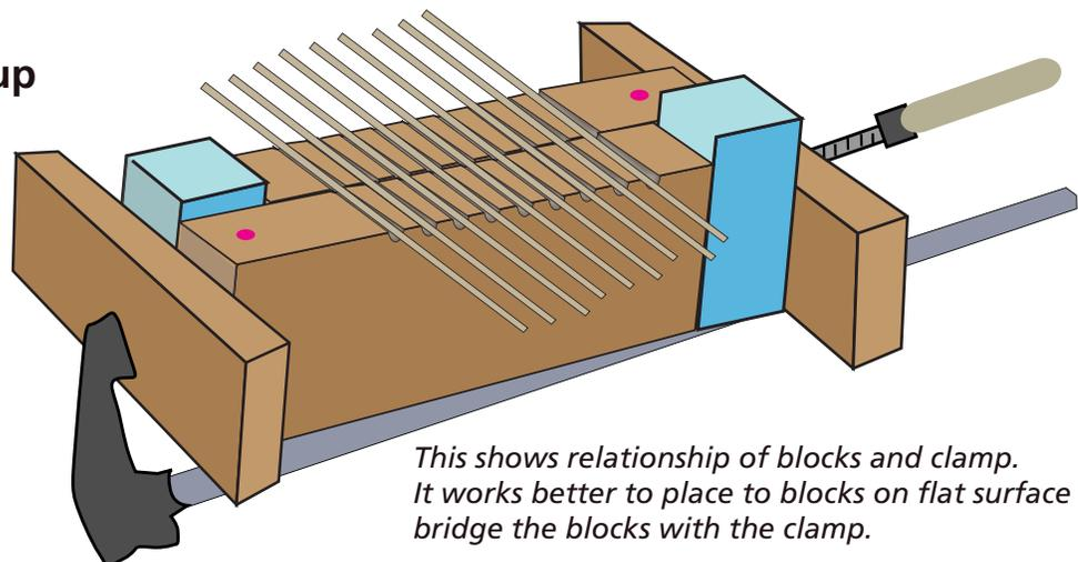
*This shows relationship of blocks and clamp. It works better to place the blocks on a flat surface and bridge the blocks with the clamp.*
